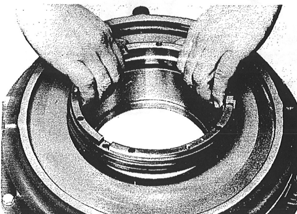
Figure 56—Removing Adapter Ring
