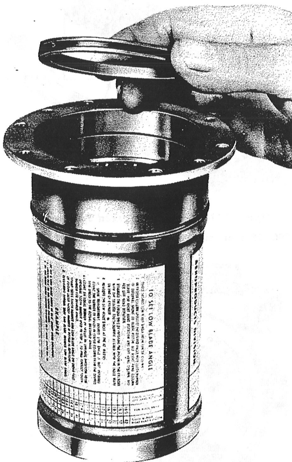
Figure 114—Installing Torque Unit Seal and Washer
